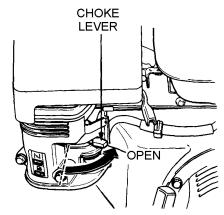
Figure 11. Engine Choke Lever (Closed)
